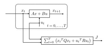
Figure 11.3.1: Finite horizon LQR realized by a block diagram.
