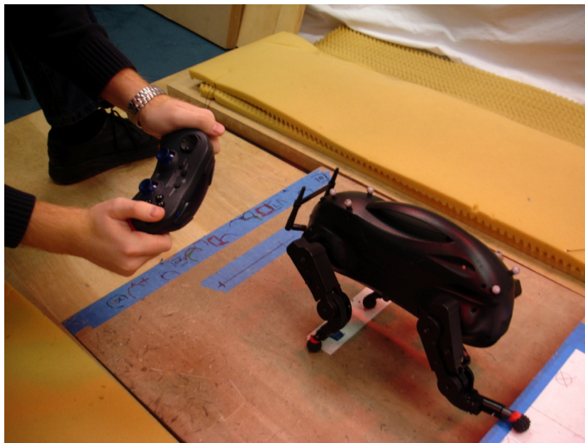
Figure 6.0.1: Human expert demonstration to train a walking robot to cross very rough terrain. Learning to Search (LEARCH) [Zucker et al., 2011, Ratliff, 2009] attempts to make a footstep planner mimic the human pilot’s choices. Imitation learning is the study of algorithms that improve decision making through data collected by observing an expert – often, but not always a person who can accomplish a task that is hard to hand-program.
