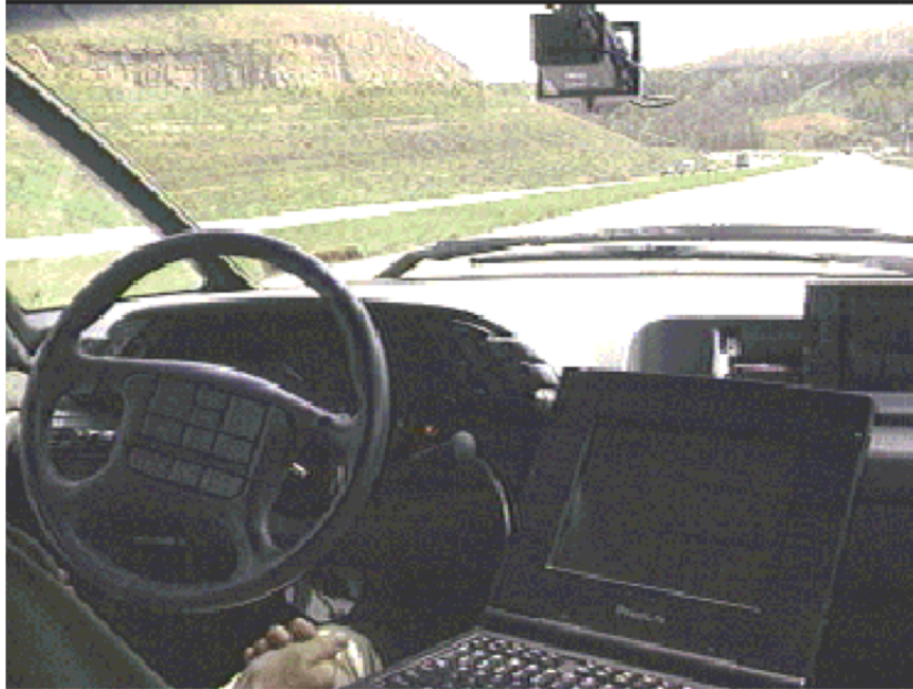
Figure 6.1.1: Pomerleau's Autonomous Land Vehicle in a Neural Network system at work driving the Carnegie Mellon NAVLAB vehicle. Used with permission.
